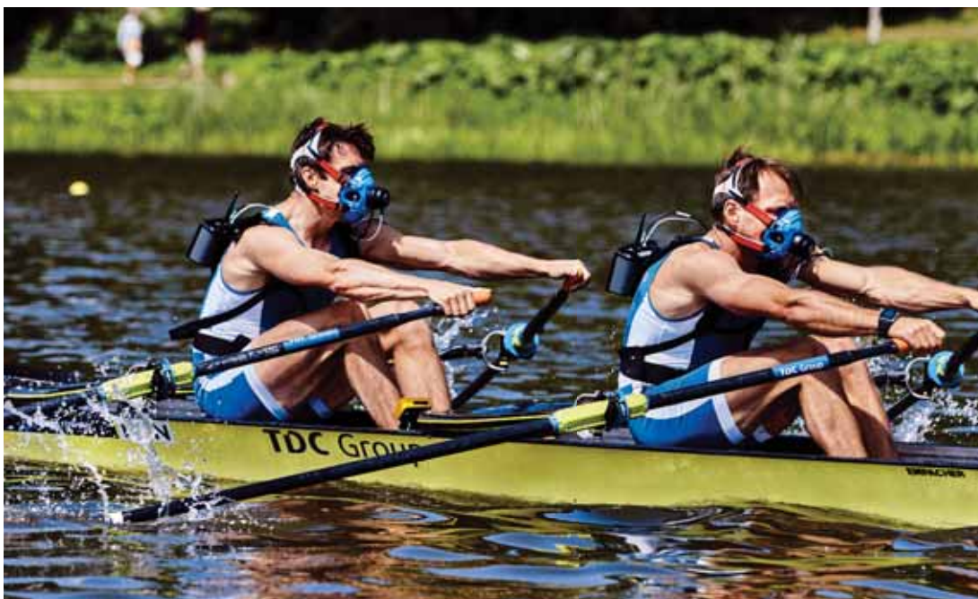
Cosmed's K5, a wearable metabolic system designed for measuring metabolic parameters both in the field and in the laboratory.
